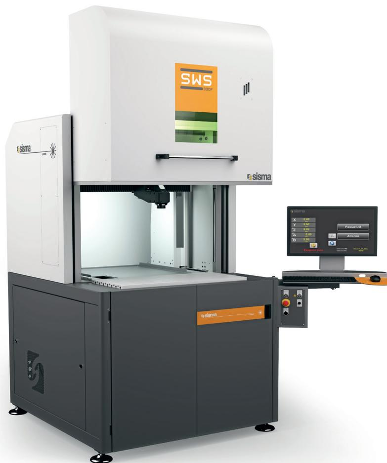
3/4 axes CNC welding station
